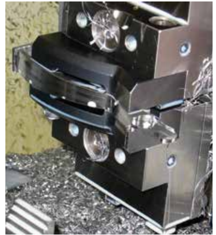
Mechanical centre-clamping vise MZS 180-80 B with custom designed jaws
