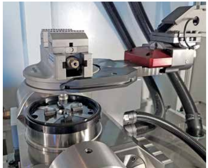
Mechanical centre-clamping vise MZQ 170-60 PA, Erowa ITS 148
