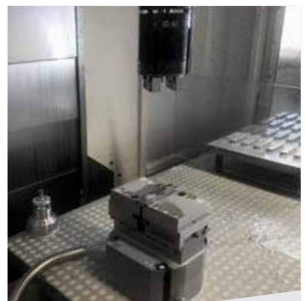
Pneumatic centre-clamping vise PZS 180-80 AT
