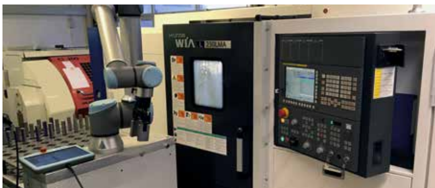
Mobile robot system SP MR 1 loads CNC lathe
